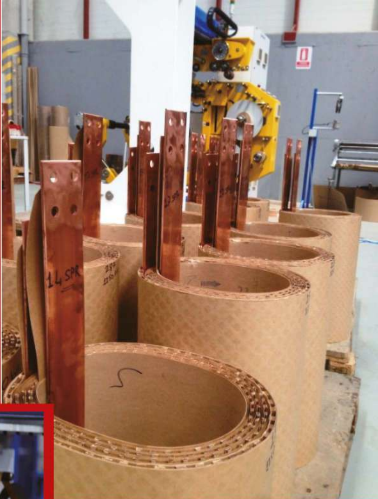
Low voltage winding
